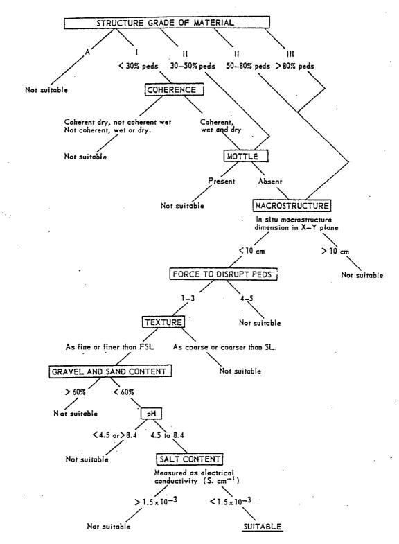
Procedure for the selection of material for use in topdressing of disturbed areas.
